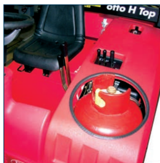
LPG systeem Installation GPL
