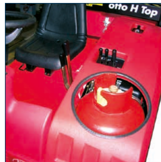
LPG systeem Installation GPL
